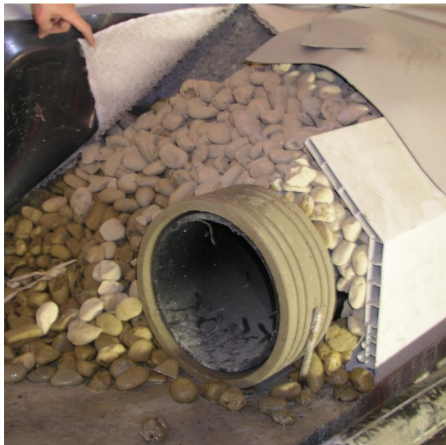
Figure 11-1 Drainage pipe, drainage gravel and prefabricated element to facilitate connection to waterproofing membrane
